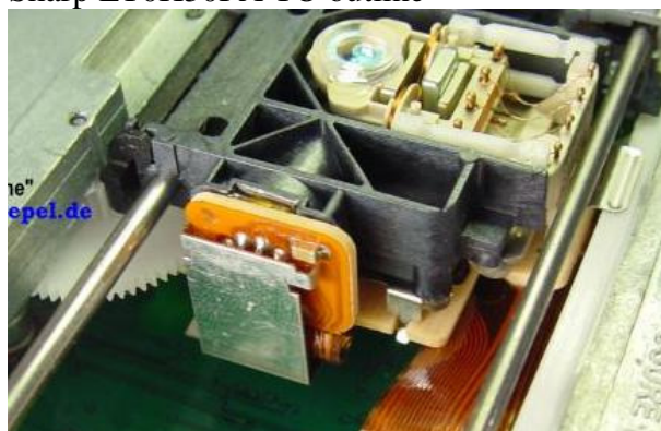
Sharp LT0H30PA TO outline and screen plate CDM12pro-CDpro2LF-VAM1254
