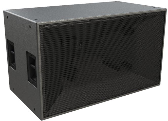
The 13 ply Baltic Birch used throughout the enclosure is encased in Polyurea for protection from impact and atmospheric conditions, and a strengthened outdoor finish is available for long term exposure to rain and sunlight. Install and touring versions of the SH96HO's are equipped with eighteen 3/8" rig points; however, touring models also include built on casters and six handles for easy movement.
