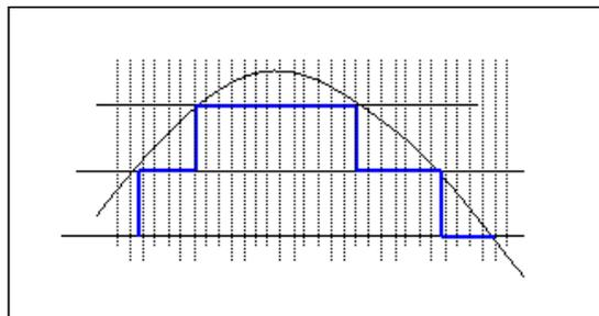
To force the linear averaging of the DAC output signal some designs use vacuum tubes or special op-amps with high power bandwidth (high gain-bandwidth product AND high slew rate!).
