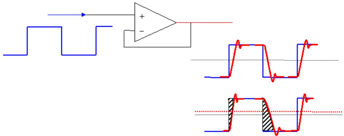
The output signal of a DAC contains a high-frequency spectrum and also a very fast settling quantized level signal. Most high-performance DA converters are settling within a microsecond. The attempt to average the DAC output signal with an operational amplifier is a challenge. Some designs use a transformer in advance of further processing to have a linear averaging and at least some low-pass filter function without the above mentioned detection phenomenon.
