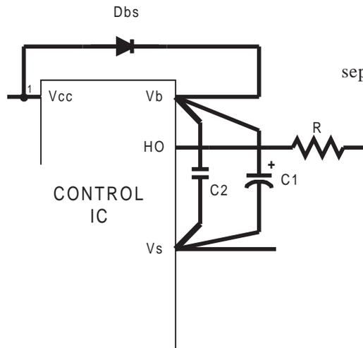
used to provide good local separate ceramic capacitor close essential if an aluminum is used for the bootstrap bootstrap capacitor is tantalum type, this in itself as the local
