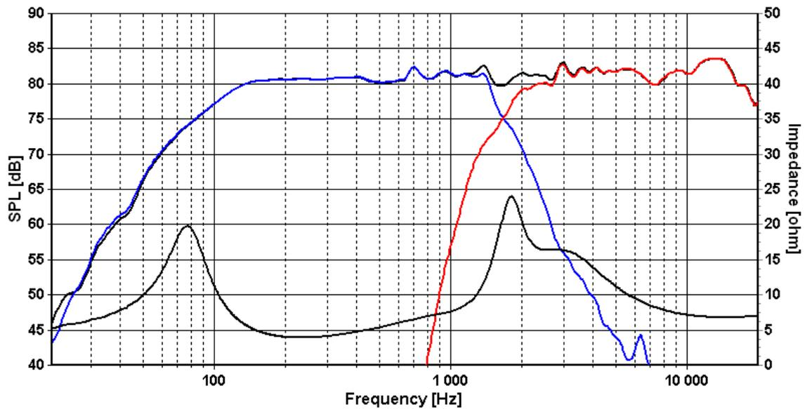
The 2nd order lowpass filter and 3rd order highpass filter result in a perfect in-phase summing of the drivers' output at the crossover frequency.
