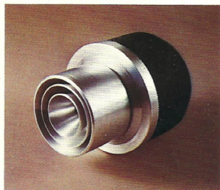
TW-1800A Horn tweeter employing 30 micron duralumin foil diaphragm. Highs extend to 20,000 Hz. Machined aluminum horn provides excellent dispersion plus natural sounds.
