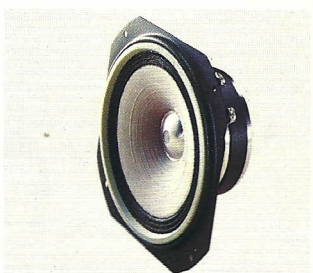
FR-12A Ideal speaker unit for compact sound systems. Provides frequency response of 80 to 18,000 Hz. Can handle up to 6.3 watts, more than ample for average listening.
