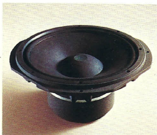
W-305A Full size 30cm woofer with new light weight cone, neoprene foam edges for frequency response extending down to 16 Hz even in compact bookshelf size enclosure.
