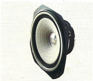
FR-16A Well designed full range speaker unit providing smooth response from 60 to 15,000 Hz. Has extra heavy duty magnet with flux density of 11,000 gauss. Can handle up to 10 watts.
