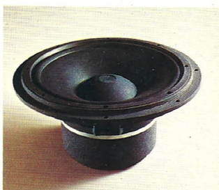
W-300A 30cm professional woofer with ferrite magnet. Capable of handling up to 60 watts. Frequency response goes down to 16 Hz, thanks to reduced mass of moving components.
