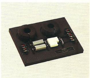
NT-600A Precision designed 2-way crossover network. Has crossover frequency of 600 Hz. Choice of 6 dB or 12 dB attenuation. Capable of handling up to 60 watts. Extra-heavy duty components throughout.
