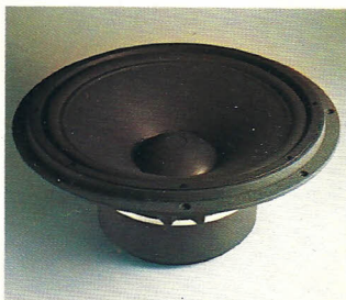
W-380A 38cm professional woofer with ferrite magnet for flux density of 11,000 gauss. Capable of handling power peaks of 80 watts. Frequency response goes down to 12 Hz.
