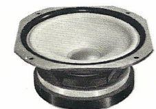
20cm (8") FULL RANGE SPEAKER 8F-60 • Impedance: 8Ω • Program source input: 40W • Frequency response: fo~20,000Hz • Lowest resonance frequency: 35Hz • Output sound pressure level: 93dB • Total magnetic flux: 175,000 maxwell • Weight: 5.2kg (11.44 lbs)
