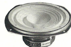
20cm (8") FULL RANGE SPEAKER FLAT-8II • Impedance: 8Ω • Program source input: 35W • Frequency response: fo~20,000Hz • Lowest resonance frequency: 40Hz • Output sound pressure level: 95dB • Magnetic flux density: 12,000 gauss • Weight: 2kg (4.4 lbs)
