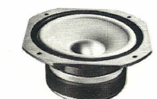
16cm (6-1/2") FULL RANGE SPEAKER 6F-60 • Impedance: 8Ω • Program source input: 35W • Frequency response: fo~20,000Hz • Lowest resonance frequency: 45Hz • Output sound pressure level: 90dB • Total magnetic flux: 170,000 maxwell • Weight: 3.1kg (6.82 lbs)
