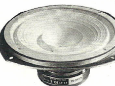
25cm (10") FULL RANGE SPEAKER FLAT-10II • Impedance: 8Ω • Program source input: 55W • Frequency response: fo~20,000Hz • Lowest resonance frequency: 35Hz • Output sound pressure level: 96dB • Magnetic flux density: 12,000 gauss • Weight: 2.8kg (6.16 lbs)
