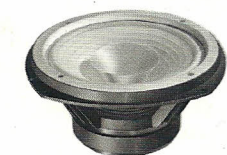
16cm (6-1/2") FULL RANGE SPEAKER BETA-6 • Impedance: 8Ω • Program source input: 30W • Frequency response: 40~20,000Hz • Lowest resonance frequency: 40~60Hz • Output sound pressure level: 93dB • Magnetic flux density: 12,300 gauss • Weight: 1.42kg (3.13 lbs)
