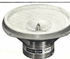
25cm (10") FULL RANGE SPEAKER BETA-10 • Impedance: 8Ω • Program source input: 20W • Frequency response: 25~20,000Hz • Lowest resonance frequency: 25~40Hz • Output sound pressure level: 97dB • Magnetic flux density: 15,500 gauss • Weight: 4.6kg (10.12 lbs)
