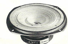
16cm (6-1/2") FULL RANGE SPEAKER FLAT-6II • Impedance: 8Ω • Program source input: 30W • Frequency response: fo~20,000Hz • Lowest resonance frequency: 45Hz • Output sound pressure level: 92dB • Magnetic flux density: 11,000 gauss • Weight: 1.4kg (3.08 lbs)
