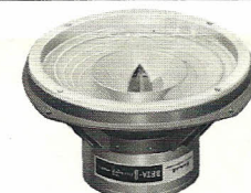
20cm (8") FULL RANGE SPEAKER BETA-8 • Impedance: 8Ω • Program source input: 16W • Frequency response: 30~20,000Hz • Lowest resonance frequency: 30~45Hz • Output sound pressure level: 95dB • Magnetic flux density: 15,500 gauss • Weight: 3.3kg (7.26 lbs)
