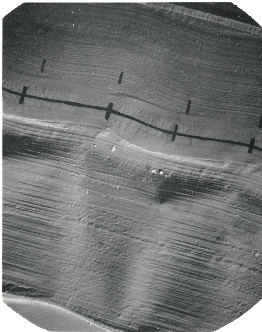
Plate 4 Electron micrograph of stereo groove (modulation as previous grooves) showing merely smoothed path of 0.0006 in. radius stylus after 250 playings at 3 gm with 0.6 mgm stylus. (The upper track—emphasized by side thrust— still shows little distortion in stylus path when compared with cutter lines.) (See pp. 31 and 37.)
