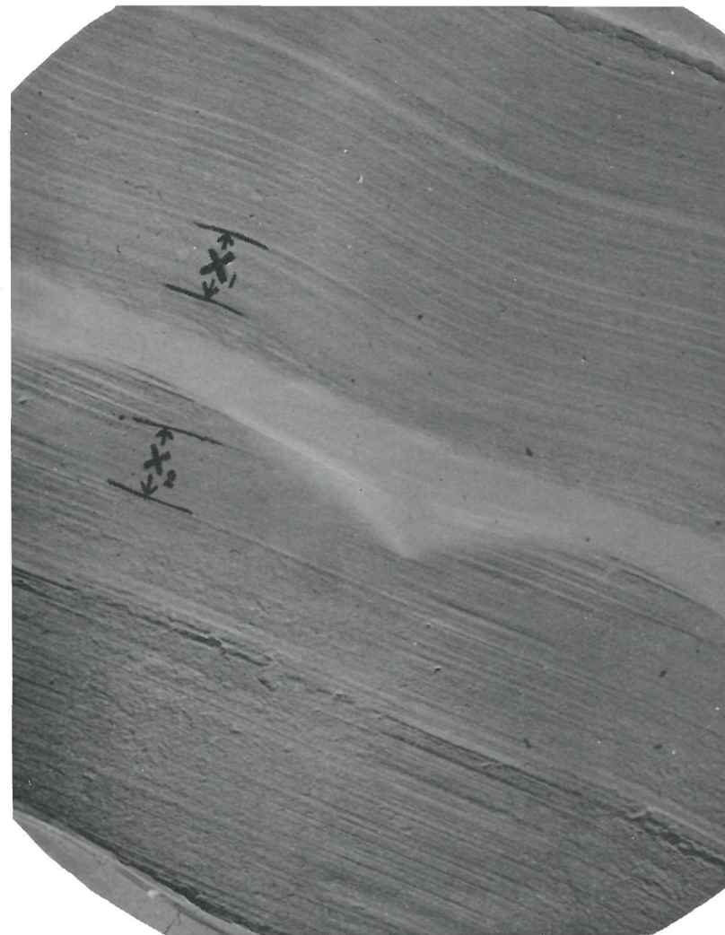
Plate 1 Electron microscope photograph (electron micrograph) of a stereo record groove after playing at 3 gm tracking-weight with a pick-up with a 0.0006 in. stylus. The groove walls show only faint impressions of the stylus path (where indicated by X^1 and X^2 ). These impressions are in the form of a slight smoothing of asperities. (In spite of the fair modulation neither is there any detectable distortion of the waveform. This is because the pick-up also has a low tip mass (0.6 mgm).) (See pp. 28 and 38.)
