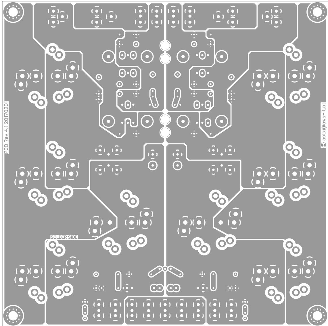
bottomassembly (mirrored), scale = 1:1.000
