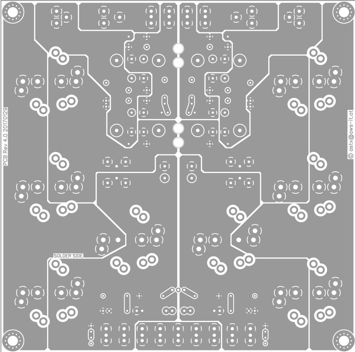
There are 8 different drill sizes used in this layout, 312 holes total
