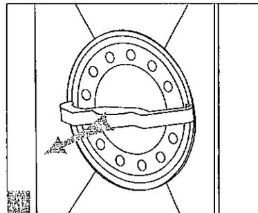
Remove the key by about 2mm. Dégager la clef de 2 mm environ.
