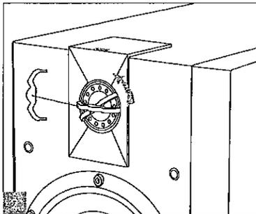
Insert the included key into the two horizontal slots. Turn the key counter-clockwise.
