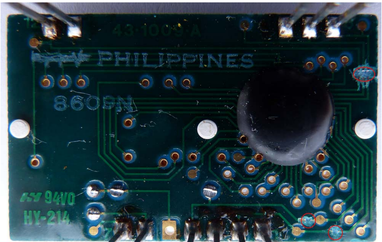
Cutting points for five tracks on the back
