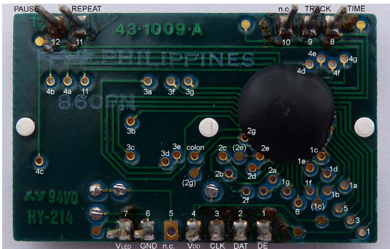
Holes (and pads) connected to each cathode and holes connected to stand-off pins
