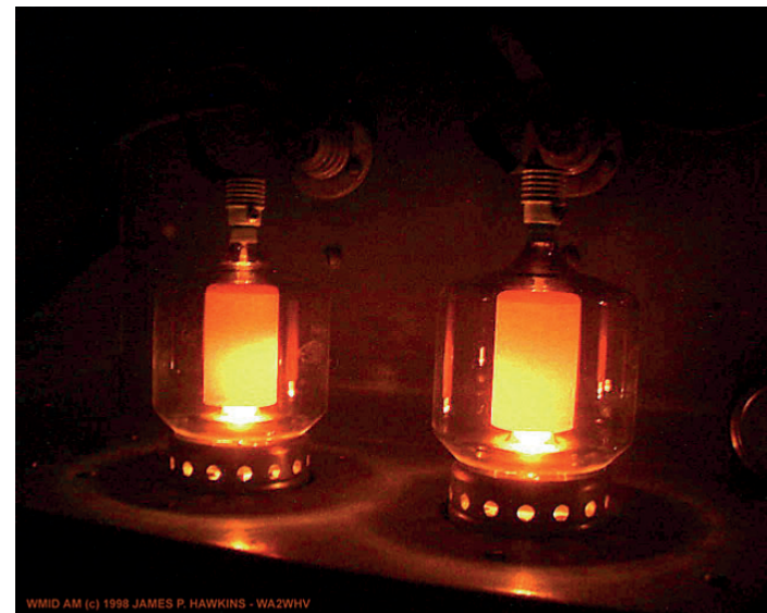
3-500Z transmitting valves undergoing stress testing. If you ever see anodes this colour there is something very wrong!
