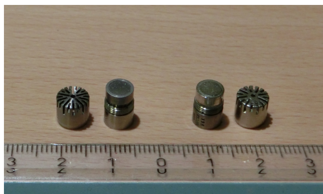
FIG. 2. (Color online) WS microphones. Left: GRAS type 40BF microphone. Right: Brüel & Kjær type 4136 microphone (equivalent to type 4939).
