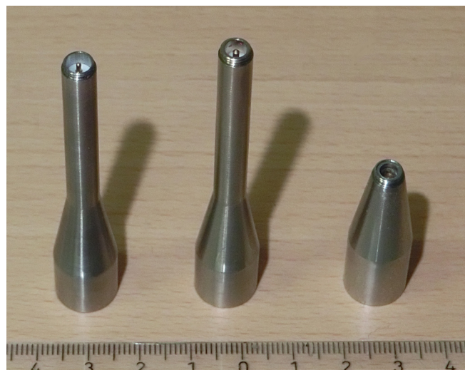
FIG. 3. (Color online) Commercial adapters for WS3 microphones. Notice the absence of shielding around the contact pin in the adapters to the left and in the middle.
