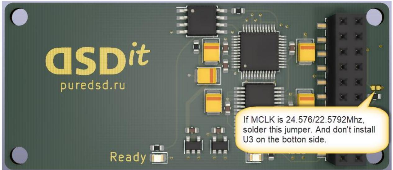
For Amanero in master mode, solder jumper. And don't install U3 on the bottom side. (work in master mode has not been tested)
