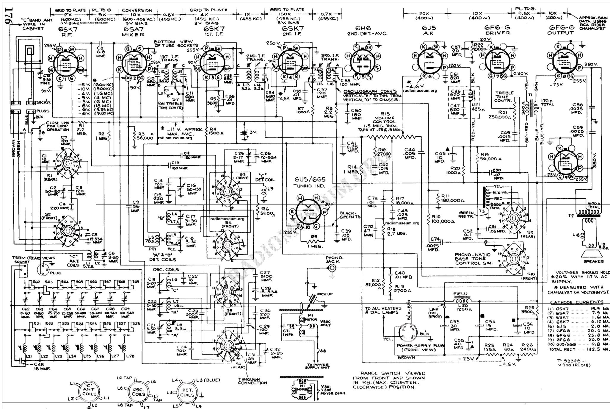
When measuring R-F and I-F gain, a 3-volt bias was connected between the A.V.C. bus and chassis, as shown in dotted lines.
