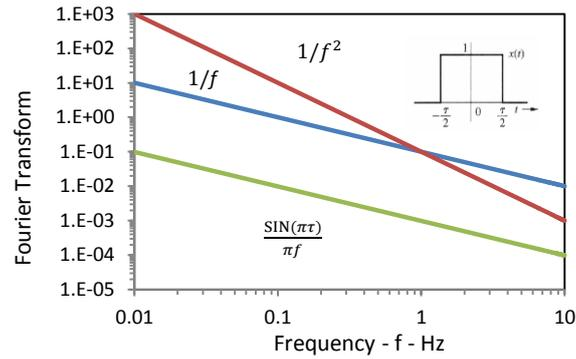
Fig. 5 FT of step change in power is shown to have the same slope as the usual  $1/f$  spectra found experimentally for LFN. The FT is based on the unit step shown in the inset. The  $1/f^2$  spectrum is shown only for comparison.
