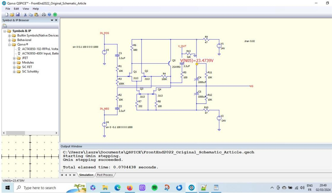
Original Schematic [with a  $10^6$  resistance load @output, done for convergence, Qspice forums], Dual Power Supply +/- 24V. Schematic on top, Voltage across C4 & C5 @bottom.
