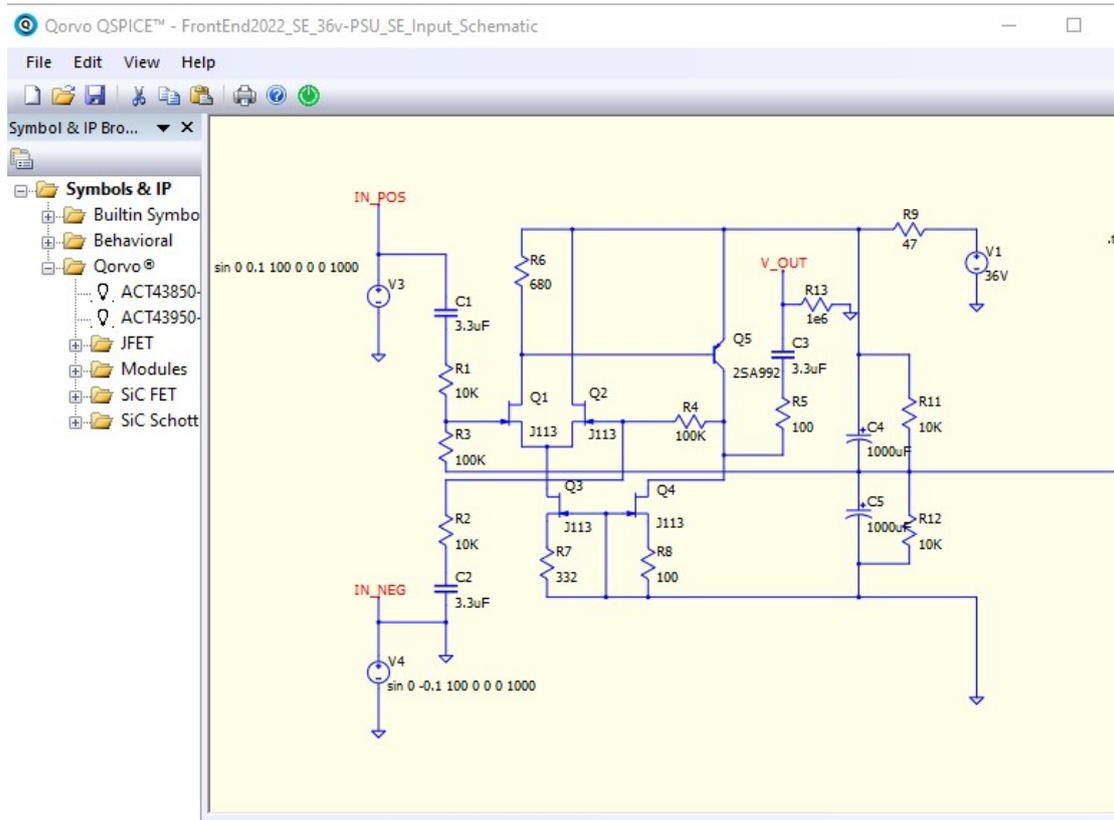
Single Ended +36V Power Supply[with a  $10^6$  resistance load @output, done for convergence, Qspice forums], Unbalanced Input (IN\_NEG to ground). Schematic on top, Voltage across C4 & C5 @bottom. (V(N04)-V(vg) across C4, V(vg) across C5)
