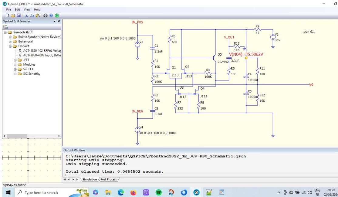
Single Ended +36V Power Supply[with a  $10^6$  resistance load @output, done for convergence, Qspice forums]. Schematic on top, Voltage across C4 & C5 @bottom. (V(N04)-V(vg) across C4, V(vg) across C5)
