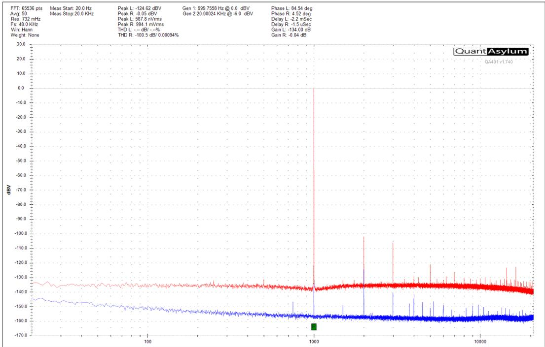
Left input to the QA401 is shorted with a 50 Ohms BNC terminator plug
