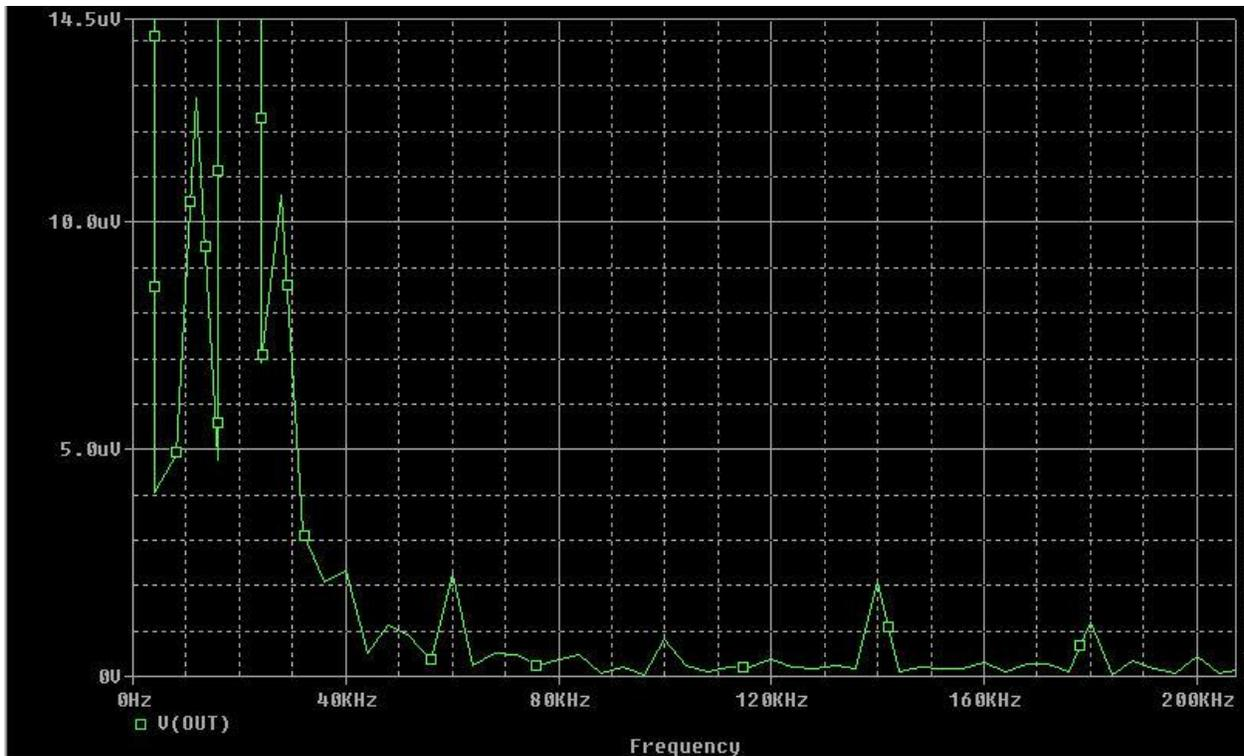
The peaks adjacent to the 20kHz fundamental are simulation artifacts (they are non-harmonic, a physical impossibility). The 3<sup>rd</sup> harmonic is now only 2uV, and so is the 7<sup>th</sup>.
