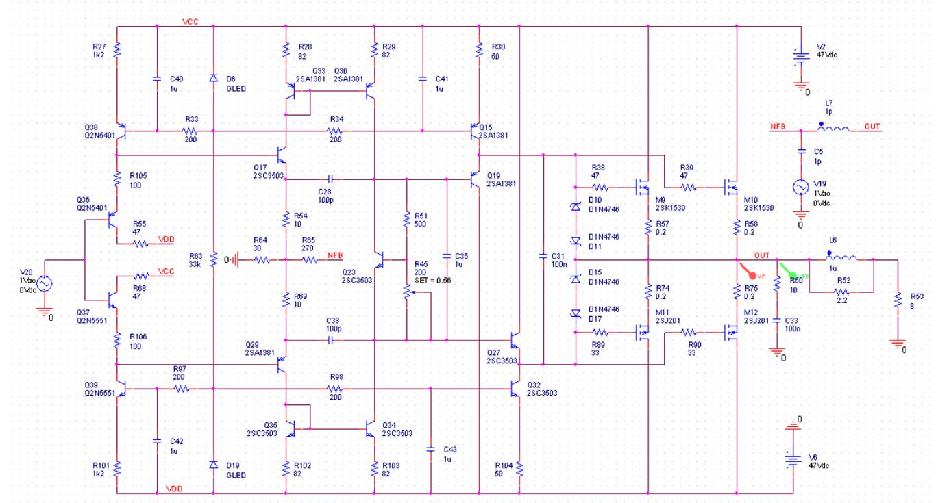
Fed at +/-47V, this output stage delivers 100W into a 8ohm load, with enough juice to support any 8ohm speaker impedance dip. The OPS gain is set to 10 by the R55/R64 ratio and it's miller compensated for a healthy 1.1MHz ULGF:
