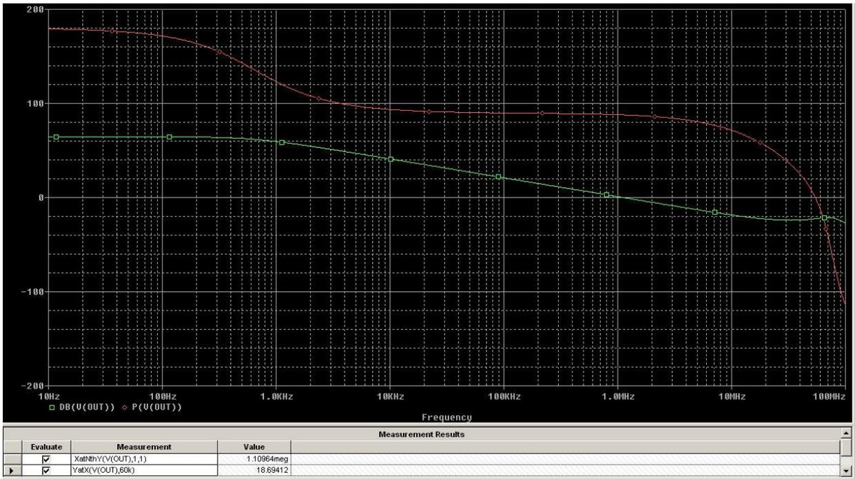
It is perhaps important to note that the OPS ULGF is NOT the closed loop GBW (that has to be much higher, to fulfill to pole-zero cancellation requirements). Here's the closed loop frequency and phase response:
