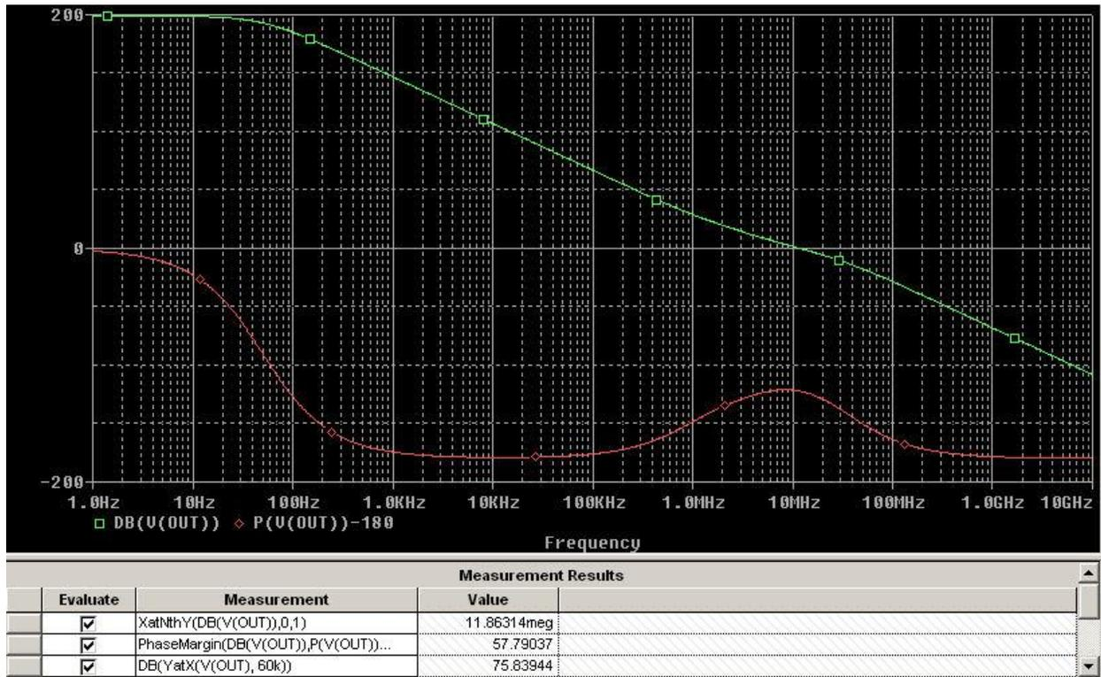
The phase margin of 58 degrees can certainly be made larger, if we can push the OPS GBW higher. But for all practical reasons, 58 degrees is good enough. Further analysis shows that for a 40V output, the phase margin is still over 50 degrees, so we should not expect any transient instabilities.
