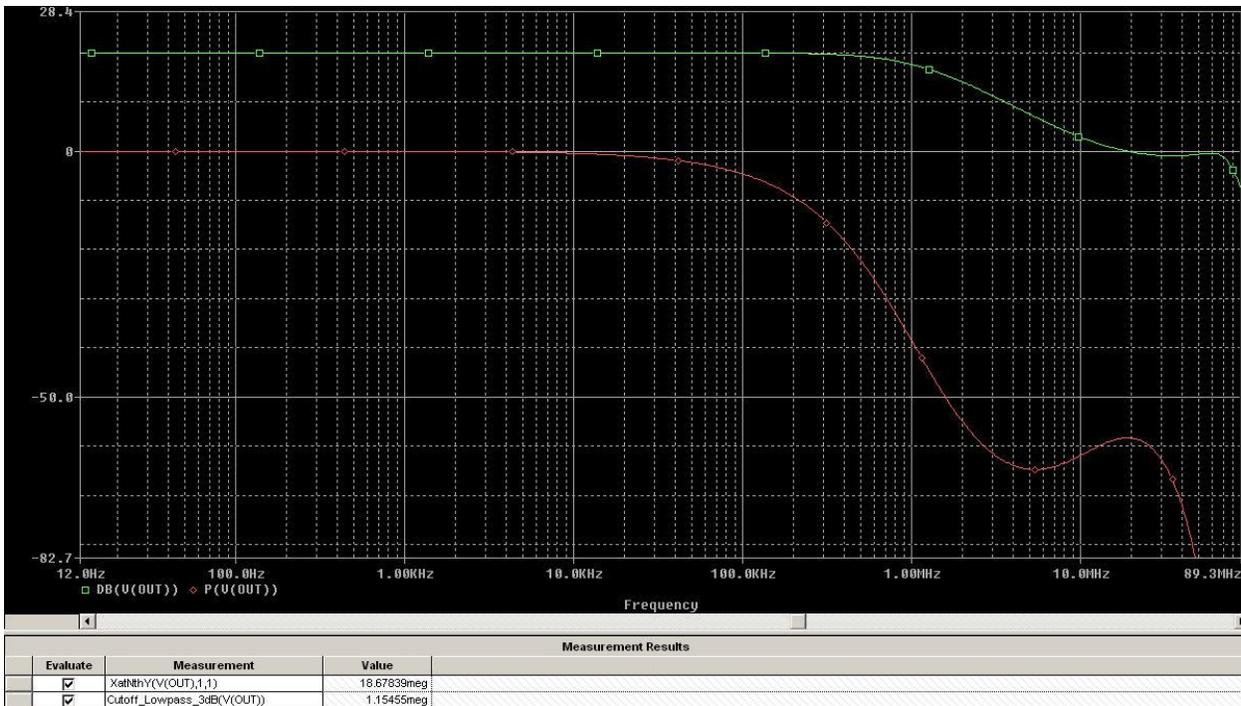
The 3dB bandwidth is 1.1MHz, while the UGF is 18.7MHz. Less than we were looking after in the previous analysis (2.5MHz/25MHz) but we'll try to fine tune to accommodate this OPS in the global feedback loop.
