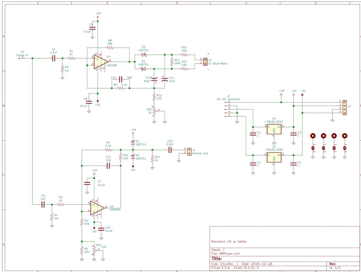
The system is powered by a 5 volt dc supply, this is labeled as +5P. A dc-dc converter will convert this to +/- 12vdc which is then regulated to 5 volts using linear regulators.
