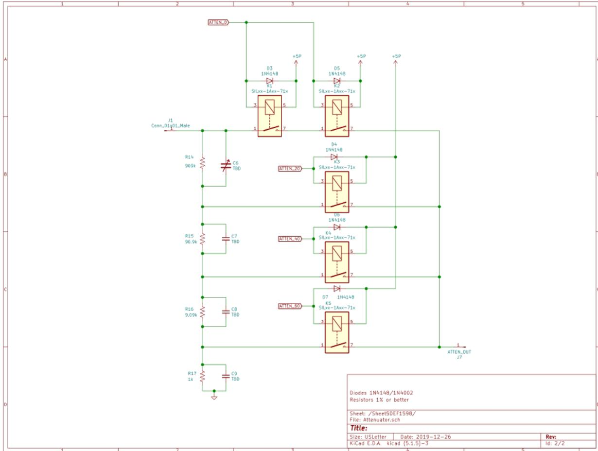
This is very similar to the original. The reed relays have a rating of 200 volts. With 100 Volts (rms) input the peak to peak value would exceed the rating and that is why there are two relays in series.
