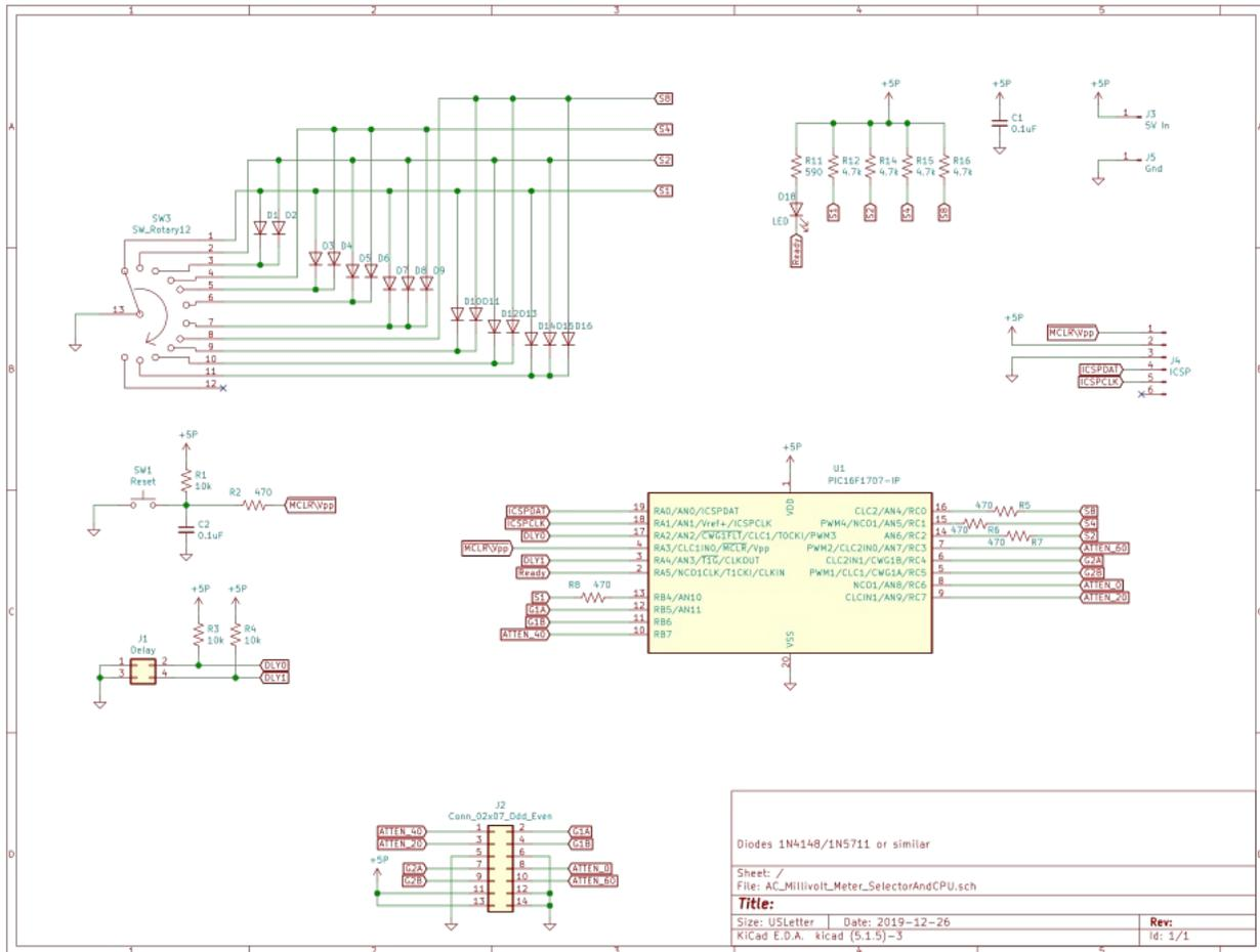
The selector has been modified from 12 positions to 11. The 300 Volt range has been removed. There is some concern about safety with a 300 Volt range and it complicated the attenuator.
