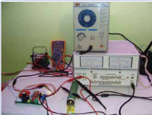
Test setup, using a audio signal generator with 0.15% THD
