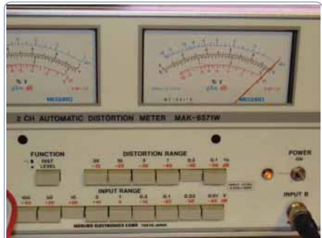
THD meter set at 0.3 % range measuring at 10 volts range.
