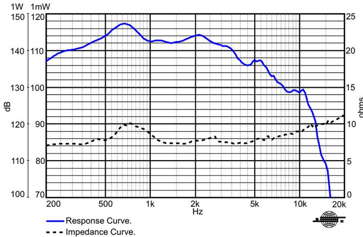
Frequency response and impedance curves measured with 50 mm terminated plane-wave tube, with sensitivity referenced to a 25 mm tube.
