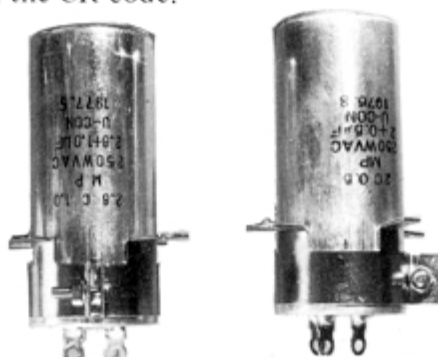
Fig. 14 MP capacitors used for crossover networks in speaker systems
