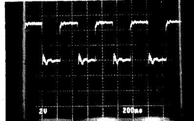
⑰ IC3-79 Pin : STOP MODE 2V/div 5μsec/div
