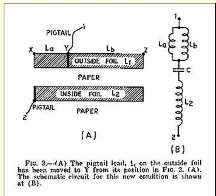
inductance designated as  $L_b$  exists between points Y and 2 of the outside foil. Under this division inductance  $L_a$  equals 1/3 of the total inductance of  $L_1$  and  $L_b$  equals 2/3 of the total inductance  $L_1$ ; likewise  $L_a + L_b$  equals inductance  $L_1$ .
