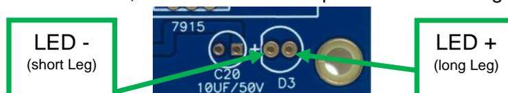
**D1 / Q9 (J112)** – Used to set bias for U1. Use the Red LED in the parts kit. Target current is 2-5mA measured across R27. Adjust R27 if necessary. Back to basics:  $V = I \times R$  Measure between 0.44V and 1.1V with voltmeter probes across R27.
