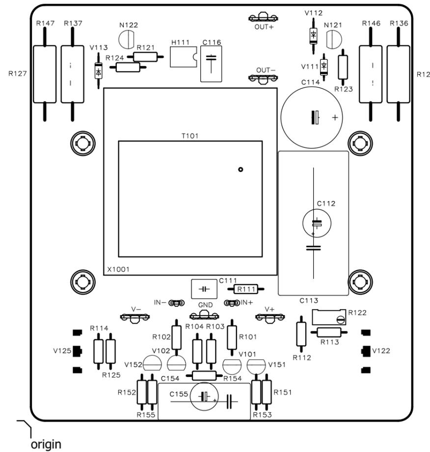
V122, V125 R126 and R127 mounted on heatsink before soldering
