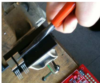
Mounting the power transistors
