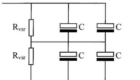
In high current applications it may be necessary to use a parallel connection. Be sure the current distribution is equal in all capacitor branches. At high frequencies, inductances can give different current distribution, as in the first illustration. In the second illustration, the distribution is equal to all capacitors.
