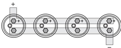
Low inductance bus bars can be built to reduce the inductance, down to less than a nH. In principle the negative side must cover the positive side.
