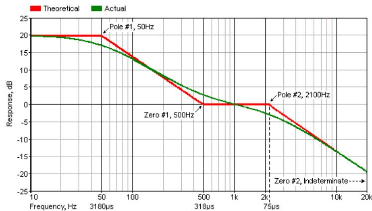
Pole #1, 50Hz:  $R_3 \times C_3 = 3180\mu\text{S}$
