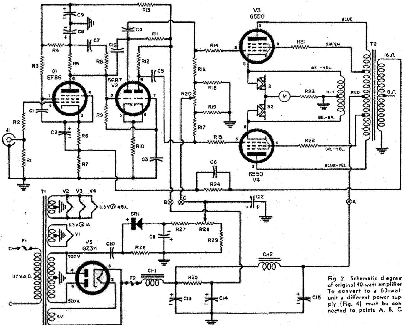
Fig. 2. Schematic diagram of original 40-watt amplifier. To convert to a 60-watt unit a different power supply (Fig. 4) must be connected to points A, B, C.
