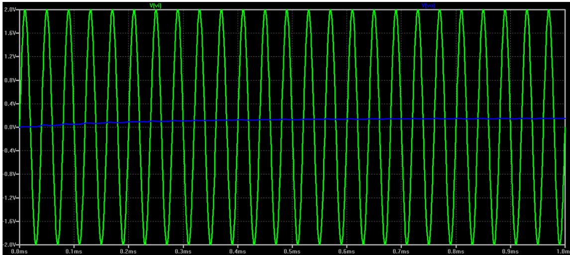
Figure 3 - Output (Blue trace) with 2V pk input at 25KHz
