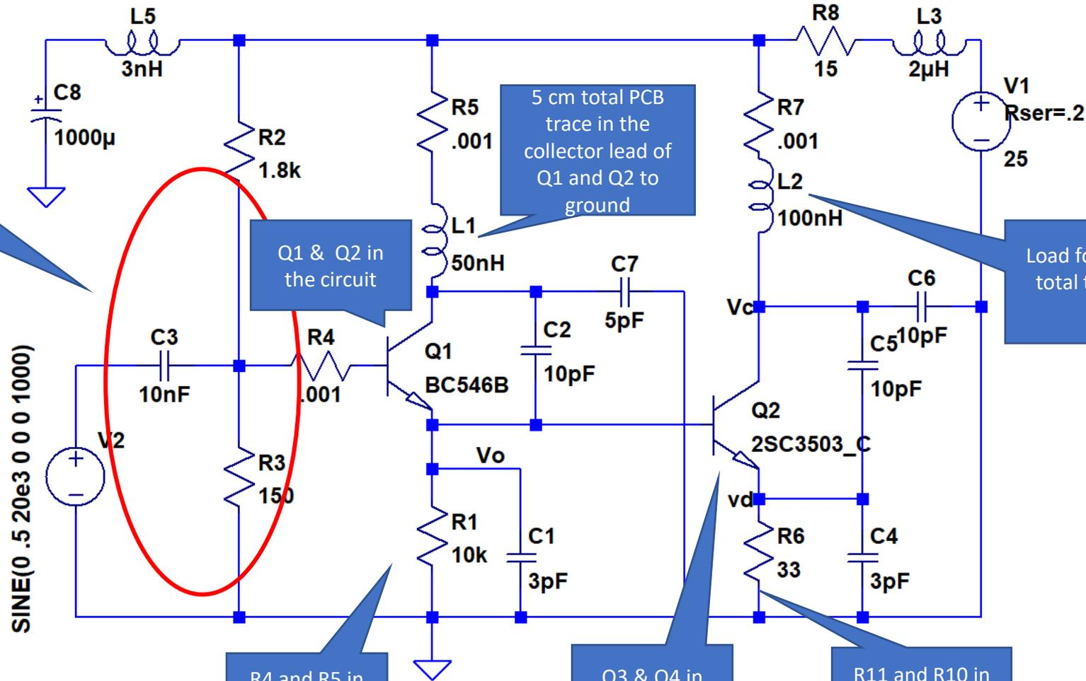
R2, R3 set up to bias output stage at about ~20mA. C3 used to move the input around
