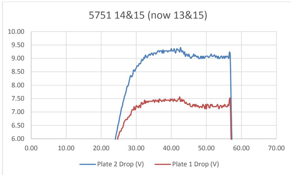
It's interesting that although plate currents of  $7.25\text{V} / 2.2\text{k}\Omega = 3.3\text{mA}$  and  $9\text{V} / 2.2\text{k}\Omega = 4.1\text{ mA}$  are appropriate for 5751s with  $-1.5\text{V}$  grid to cathode and  $250\text{V}$  plate voltages they're "off the charts" for 12AX7s (albeit with  $6.3\text{ VRMS}$  heaters)!
