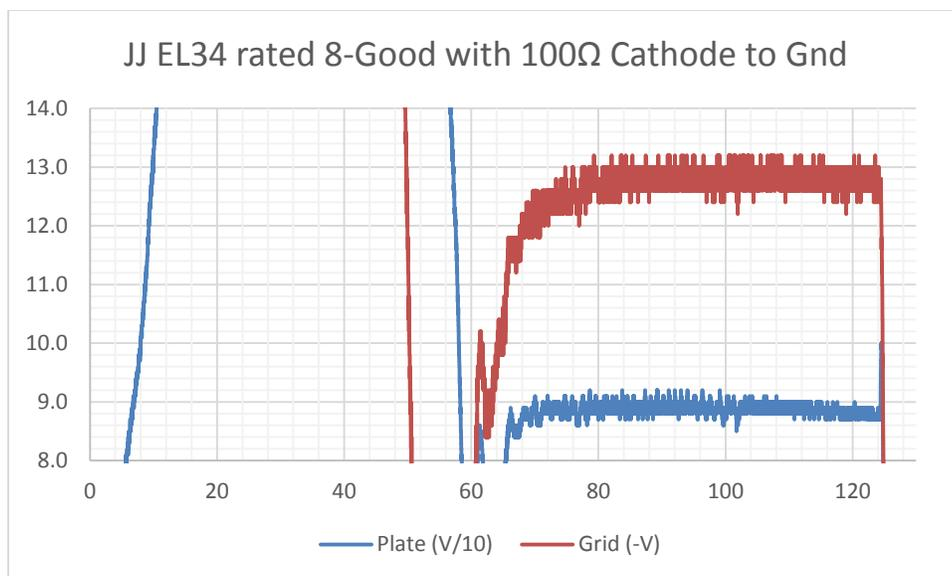
13. Unless the VT1000 is allowed sufficient time to cool down after this type of test, it will terminate testing early and “Fail” the tube; as can be seen in the following data charts for a fresh “matched” EL34. So, the VT1000 can’t be conveniently “tricked” into “rating” power tubes at a higher cathode current!
