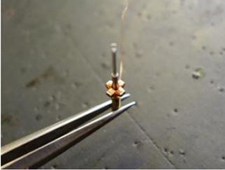
The above photograph is coils used in a typical MC cartridge. This vibrates more than 20000 cycles in a second. It is natural to think that lighter weight is better for the faster motion. Optical cartridge has the same cantilever as MM/MC. However, it has no coils nor magnets. It has only a tiny slit plate of 50  $\mu\text{m}$  in thickness. Lighter moving parts for better frequency response. This is another advantage of Optical cartridge.
