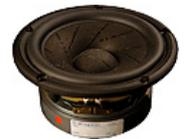
The long-stroke bass/midrange driver has a total throw of 20 mm which makes it capable of moving more air and generating more bass output than most 6 1/2" woofers. The special linear spider exerts no additional force even at maximum cone excursion. This allows the unit to respond with extreme precision to dynamic variations.
