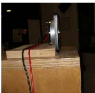
The speakers are mounted on test casing
