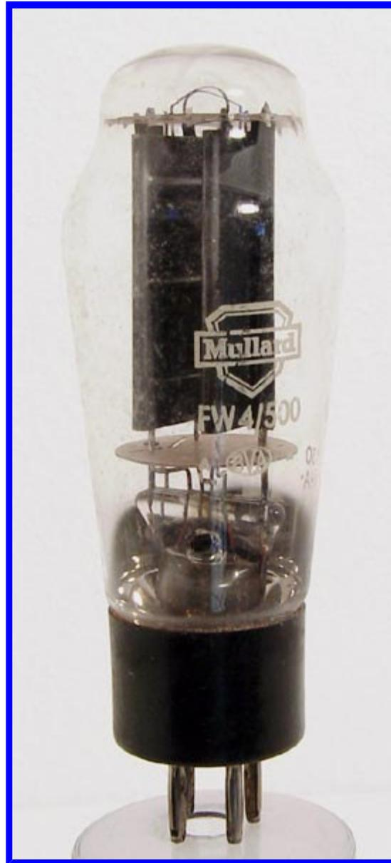
The FW4/500 full wave rectifier is a higher power device than most full wave rectifiers at 500 Volts at 250 mA. The valve is directly heated. The maximum reservoir capacitor is 16  $\mu\text{F}$  and the minimum effective series resistance has to be 200 Ohms.
