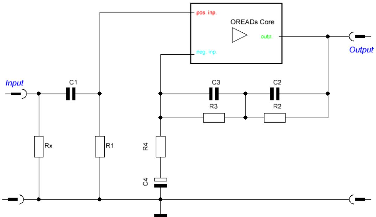
At first glance we recognize two inputs and a common output, the "negative input" is fed by the "positive output" of the actual amplifier (the term positive refers to what happens at the other input, which we use for level control - as the MM pickup input), this is generally called feedback as we know.
