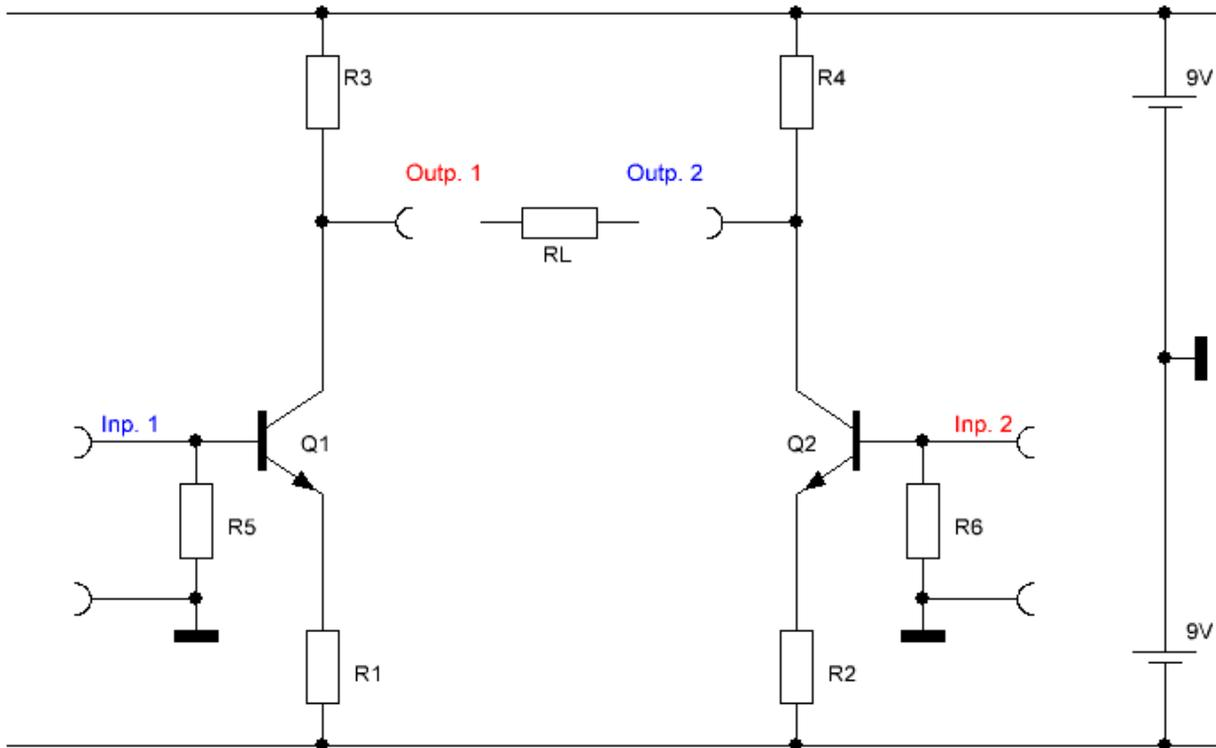
The base potential is automatically greater than the emitter potential (the voltage of the respective electrode in relation to the reference, the zero voltage at the point we call ground or earth), i.e. Q1 & Q2 are in a conductive state and currents are flowing.
