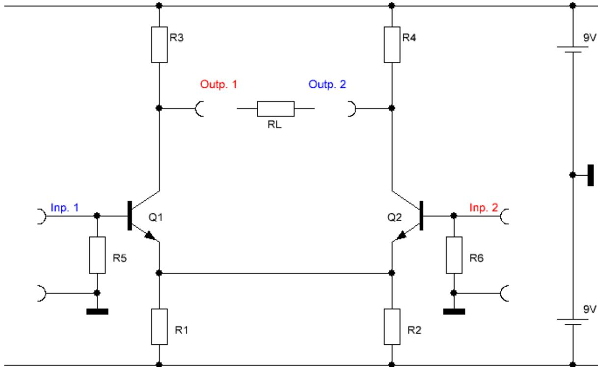
For Q2 is Q1 now working as a impedance converter, an emitter follower that wants to communicate something to its emitter electrode. For Q1 is Q2 a further processing stage, an amplifier in a so-called base-circuit.
