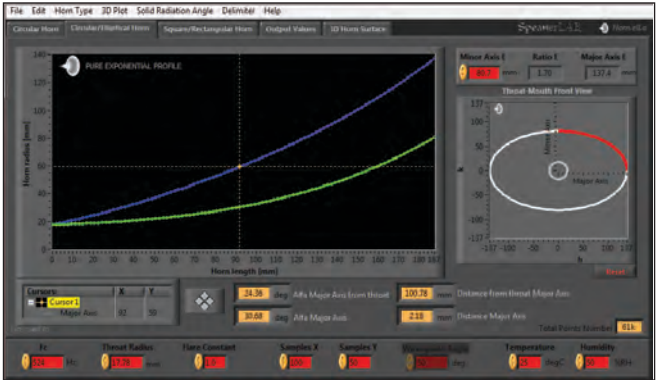
Figure 18: Elliptical mouth horn's arrangement. MR = 1.7
