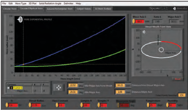
Figure 19: Elliptical mouth horns arrangement. MR = 2.4
