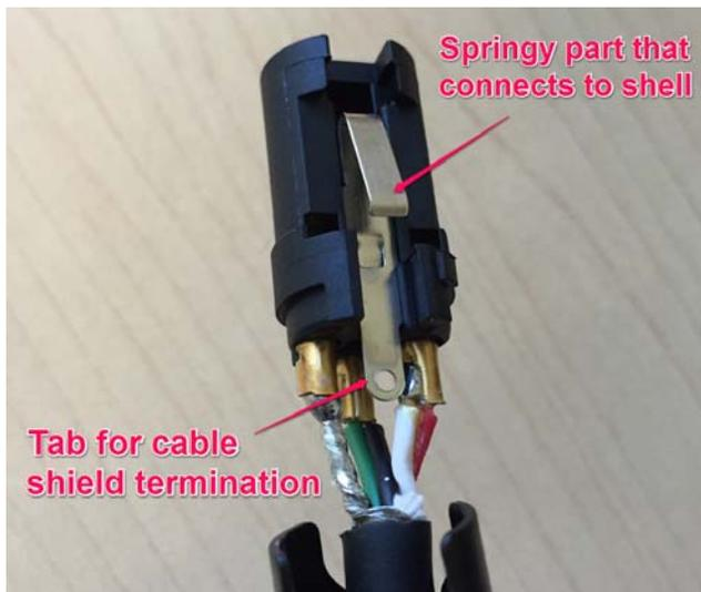
The point of this component, which is part of the original XLR specification, is to provide shield continuity to the cable connector's metal shell:
