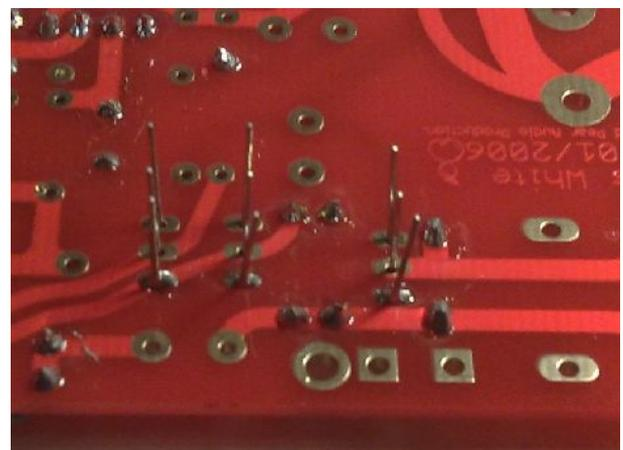
Hold the LM318 in place with a finger (pay attention to the right orientation!) and solder two of the pins, like in figure. Now you can solder all other pins without worrying of the LM318 going around...
