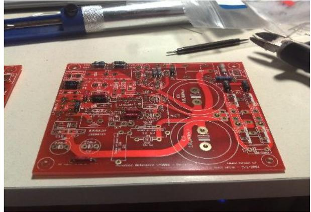
So we'll start with 1/4W resistors and we proceed then with 1N4001 and SBYV27 diodes
