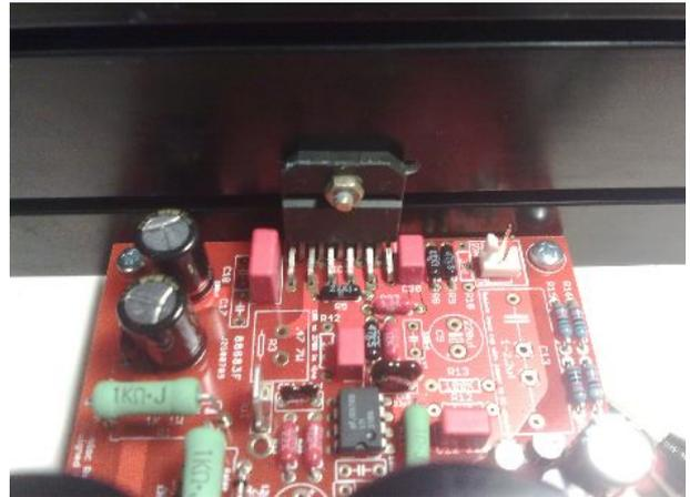
Now insert the LM3886 with heatsink to the PCB, solder two pins on the top. Remove heatsink, turn the board and solder all LM3886's pins. Use the same heatsink for the other monoblock too, so they're identical and you can use any of them to sign hole's position to the other heatsink.
