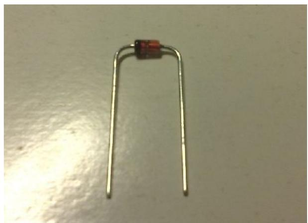
Now we're going to prepare Zeners for mounting. With help of a little screwdriver bend leads so that we have the diode like in the figure.
