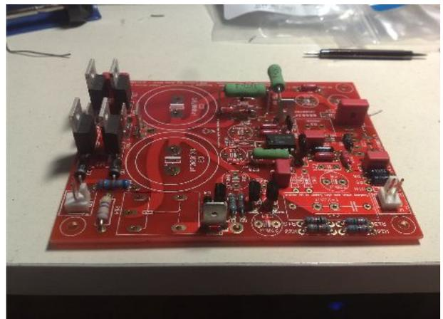
It's the rectifiers turn. Put one at time in place and, while the diode is straight, solder one leg on the top side, like in figure. When you've done it for all four diodes turn the PCB and solder the diodes.
