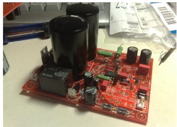
Hold the relay in place with a finger and solder two opposite pins. Turn the board and solder all remaining pins.
