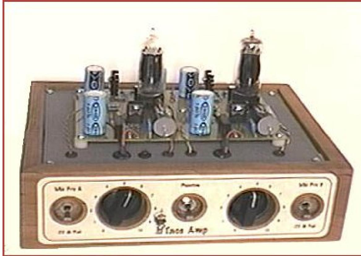
Here is the separate power supply, a small transformer for phantom power is inside the case.
