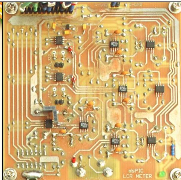
**Fig 4 : Analog Stage Board - Top.**
