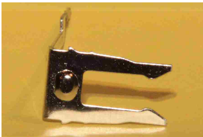
Photo 11: "Forks" of the factory RCA socket
