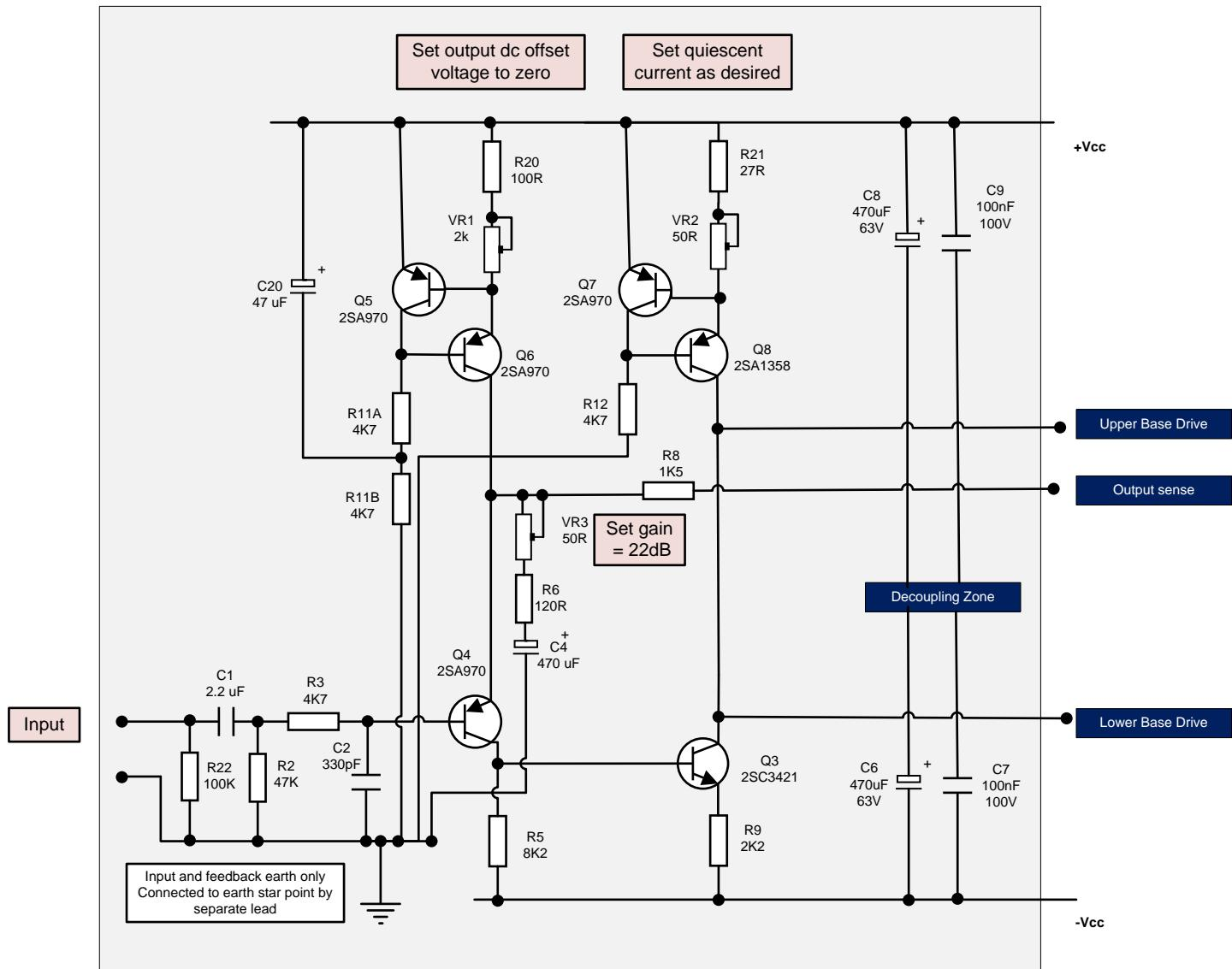
Geoff Moss' JLH, Driver Board with additional stopper resistors on preset pots,
