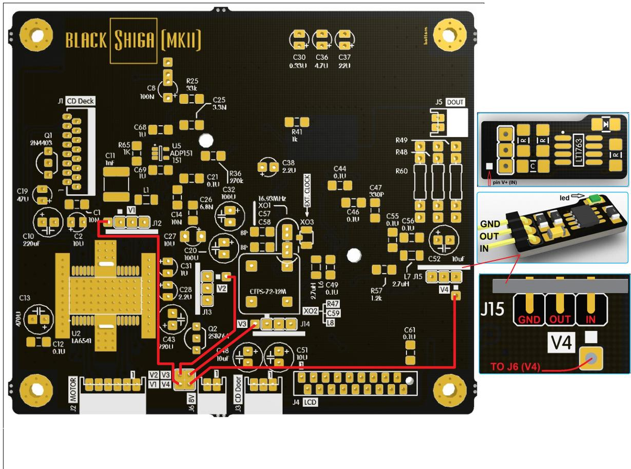
And for each mini-reg in use you should remove the correspondent ferrite bead:
