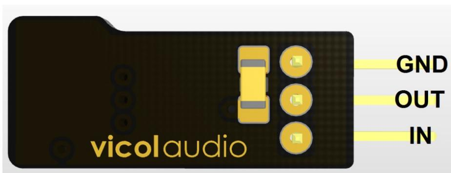
Picture below describe how to mount all 4 mini-regs. First insert each mini-reg as seen, taking pin V+ / IN as reference. Then use a small cable to link each mini-reg to 8V+ (near J6).
